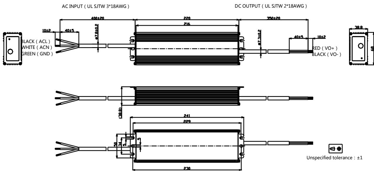
Note: Please make sure the output cable does not connect to dimming cable or the cables of other drivers until 20 seconds after being tested because of the remained voltage in the output capacitor.
