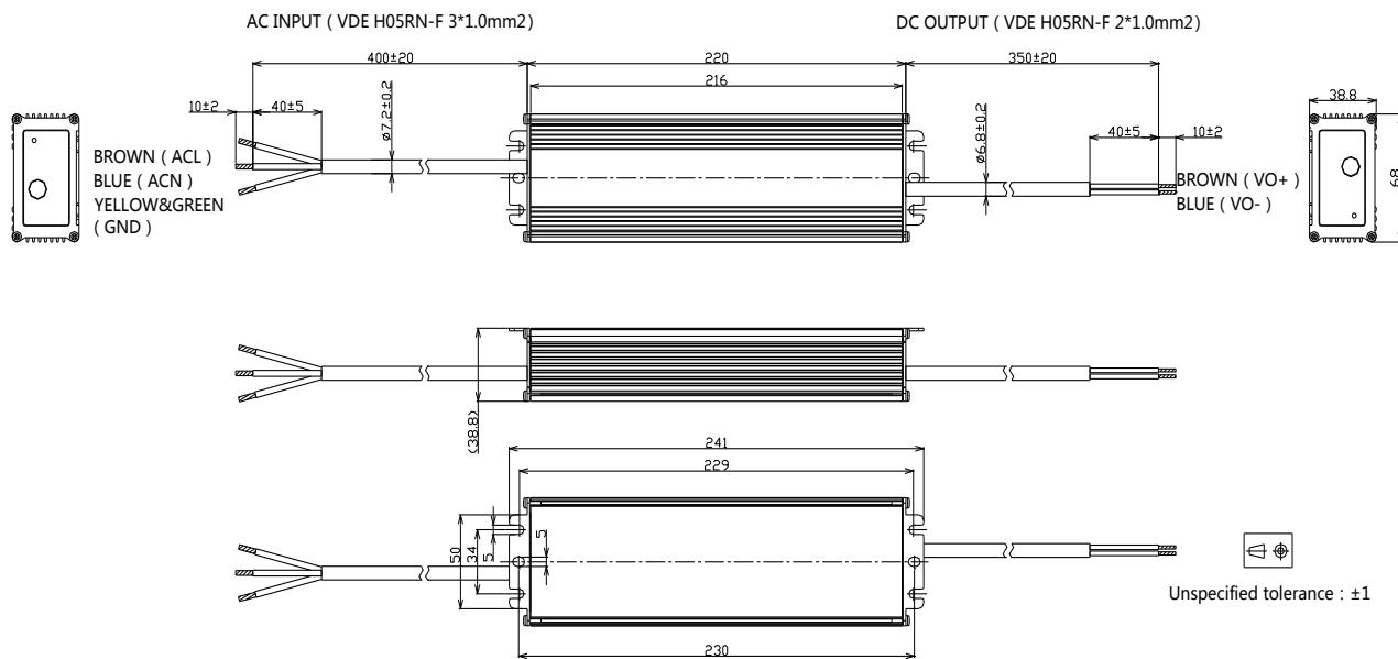
Note: Please make sure the output cable does not connect to dimming cable or the cables of other drivers until 20 seconds after being tested because of the remained voltage in the output capacitor.
